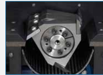
Knives holder and gearbox secured with conical expansion bushings
