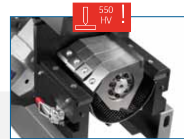
Grinding chamber in standard antiwear configuration
