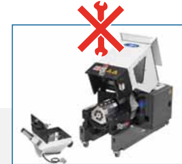
Opening by only three quick release clamps and one microswitch
