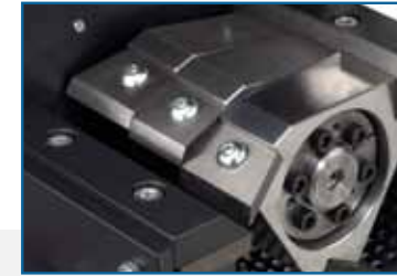
Disposable knives fixed with a single screw; adjustable counterknives
