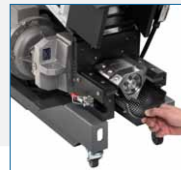
Knives, counterknives and screen in standard antiwear configuration
