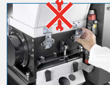
Main maintenance parts accessible without tools
