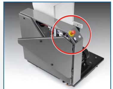
Integrated electrical control panel
