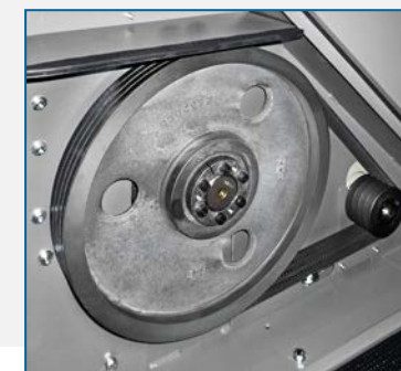
Flywheel and pulley mounted with taper-lock bushing
