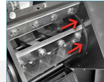
Rotor equipped with lateral discs
