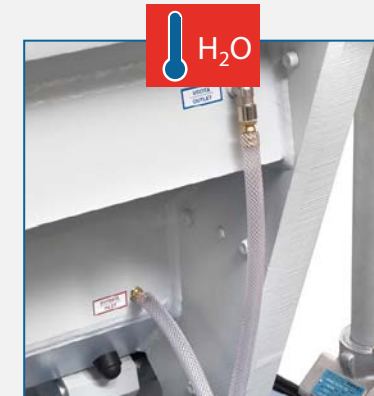
Water cooled cutting chamber
