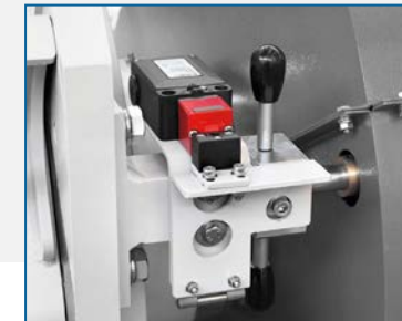
Rotor lock device for maintenance
