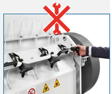
Main maintenance parts accessible without tools
