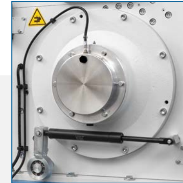
Screen cradle motion support by gas cylinder
