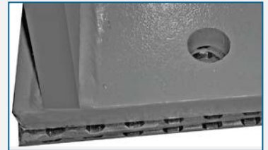
Base set on vibration dampers
