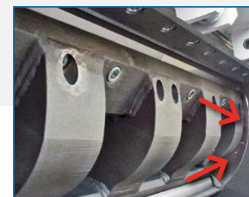
Rotor equipped with lateral discs Optional: Discs fixed to the cutting chamber
