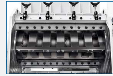
7-knife rotor with arrow-cutting configuration
