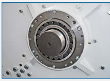
The use of spherical roller bearings that are directly mounted to the cutting chamber in cast iron housings ensure longevity of the machine
