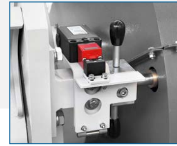
Rotor lock device for maintenance
