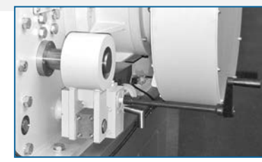
Opening of screen holder by manual jack
