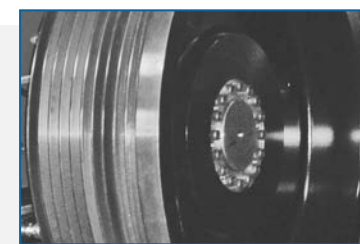
Flywheel and Pulley mounted with taper-lock bushing
