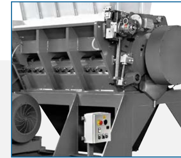
Motorized jack for hopper opening; integrated electrical control
