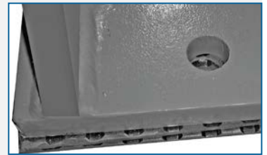
Base set on vibration dampers
