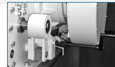
Opening of screen holder by manual jack
