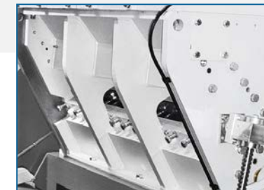
All cutting chambers can be offered in an antiwear configuration. This includes the lateral discs, the wear rings and the screen
