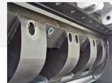
Rotor equipped with lateral discs Optional: Discs fixed to the cutting chamber
