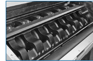
6-knife rotor with scissors-cutting configuration
